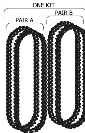
**NOTE: DIAMOND CHAIN WILL SUPPLY THE FULL KIT OF COMPONENTS THAT WILL PROVIDE FOUR CHAINS FOR ONE COMPLETE INJECTOR UNIT AS SHOWN ABOVE. THE CHAINS WILL BE SUPPLIED LOOSE, TO BE ASSEMBLED BY THE USER.**
