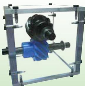
Installment : Nonparallel and nonintersecting gears
