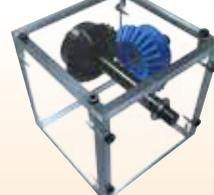
Installment : Intersecting axes gears
