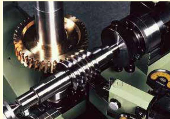
Worm gear testing machine by Klingelnberg
