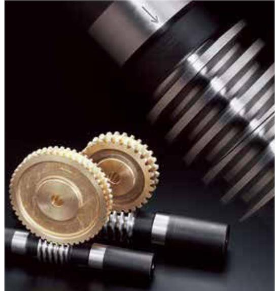
An arrow marking on the outer circumference of the hub of the KHK duplex worm indicates the direction of assembly as well as acts as a guide for the backlash adjustment. When the worm is held with arrow mark pointing right, the tooth thickness is thinner on the right and thicker on the left. Therefore, moving the worm to the right causes the thicker teeth to come into actual engagement with the worm gear, thereby reducing the backlash. (Fig.2)
