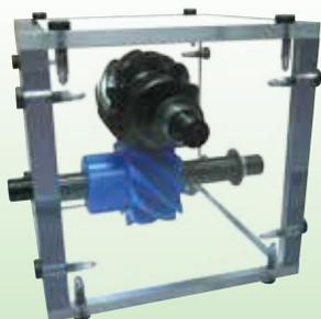
Installment : Nonparallel and nonintersecting gears
