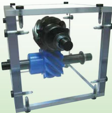
Installment : Nonparallel and nonintersecting gears
