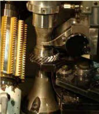
Gear cutting by a Hobbing Machine
